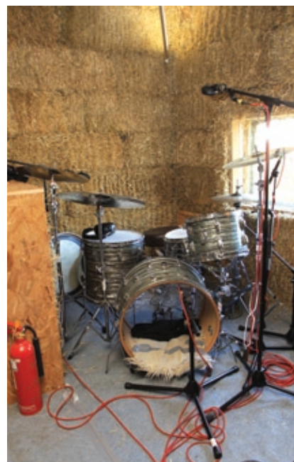
A 'Glyn Johns'-style miking technique was employed throughout on the drums, with Coles 4038 ribbon mics as the main overhead pair.
